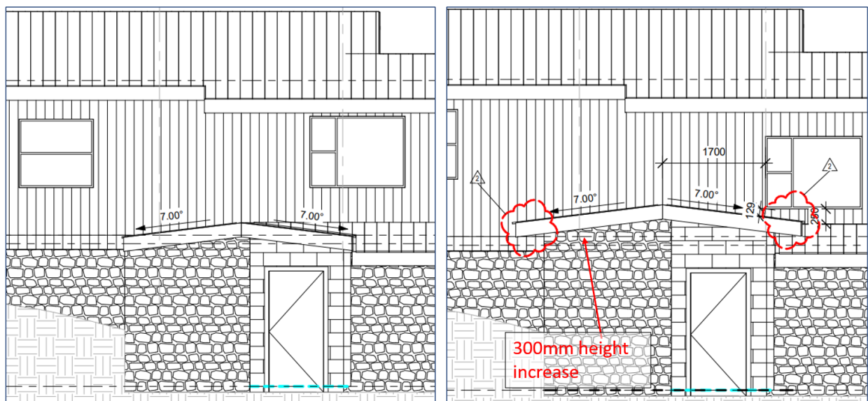
Figure 2 | Elevation plan identifying the 300mm increase in height of the entrance-way gable roof (Source: Applicant's Modification Application 2023)
